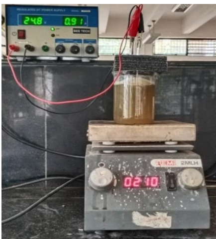
Fig. 5 Laboratory Electrocoagulation setup
